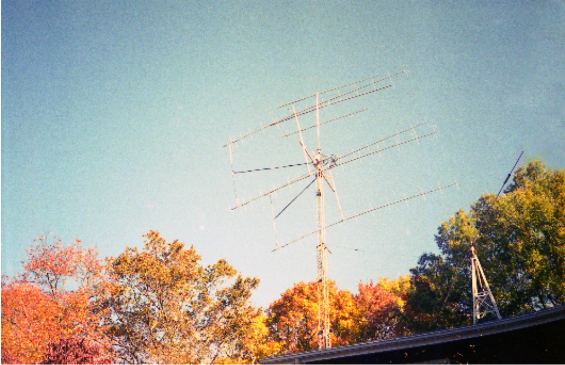
Dual-polarization 4-yagi array at K1JT, with beautiful fall colors in the background. Single yagis for 50, 222, and 432 MHz are atop the EME
